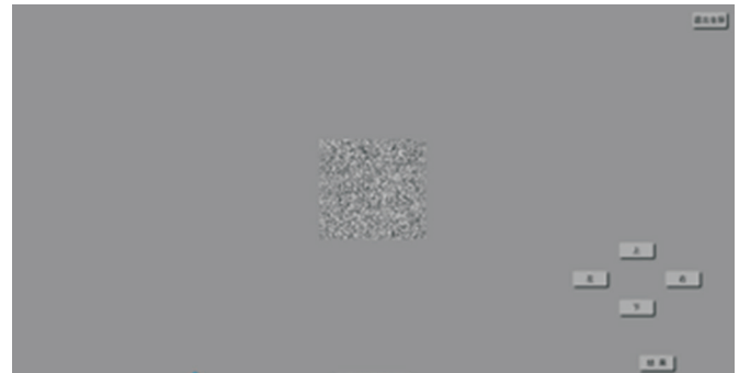
Figure 3 Example of zero-order test (in the view without 3D polarized glass) With 3D polarized glass and monitor, normal subjects would observe a stereo “E” with different orientations.
